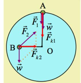
$$SF = F_{k1} = mW^2 R \rightarrow F_1 + mg = mW^2 R \rightarrow W = \sqrt{\frac{F_1 + mg}{mR}} \rightarrow$$
